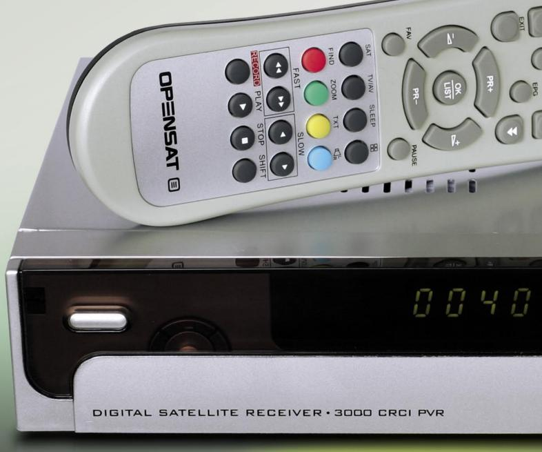
If you open this flap it reveals seven buttons to operate the receiver without remote control, a CI slot for all standard modules like Irdeto, Seca, Viaccess, Cryptoworks or Nagravision, a Conax card reader as well as a USB interface.
